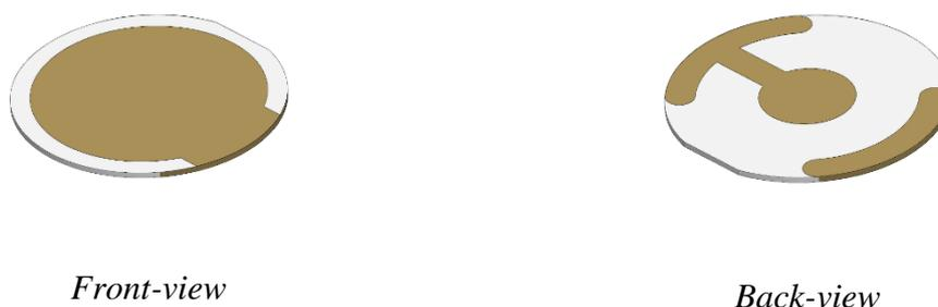
**Fig. 2.4:** Structure of a QCM resonator.
