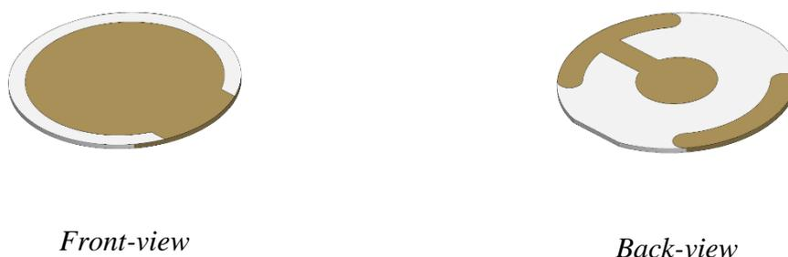
**Fig. 2.4:** Structure of a QCM resonator.
