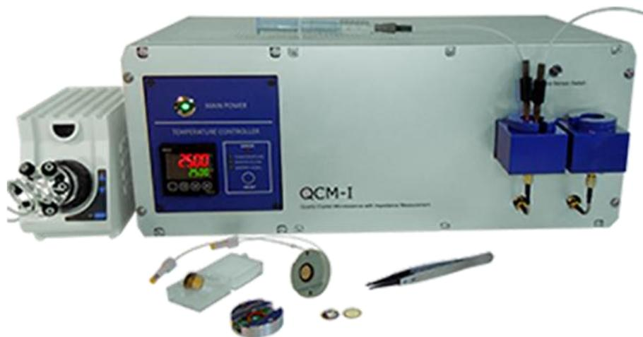
**Fig. 3.5:** QCM-I 008 unit setup (Courtesy of MicroVacuum Ltd).
